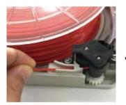
Insert the filament between the rollers.
