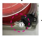
Place the filament into the feeding hole.
