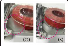
Make sure the refill filament is placed properly as shown in the image above.
