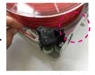
Make sure that the filament has been inserted to the tube properly.
