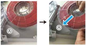
Place the refill filament in a diagonal direction so it won't push the part (A).
