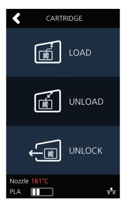
For 10 seconds [LOCK] states is deactivated and the user can detach cartridge from printer. \*If the cartridge can't be pulled out even after "unlock", gently push it forward and then try to pull out again.
