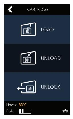
When **[OK]** is pressed at the cartridge unload confirming message, Cartridge unloading will automatically proceed. To remove filament, the nozzle is heated up to the specified temperature and the filament unload starts.
