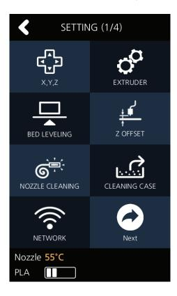
On the SETTING page, user is able to perform bed leveling. The bed leveling process consists of 3 steps. From the center, the top side is measured first, and then both sides of the bottom level are measured. If the height of the bed is perfect then levelling process will be finished but if the height of the bed and nozzle does not match, screws will appear informing user the direction and the number of clicks(angle) of screw rotation.
