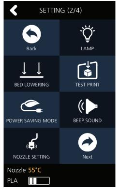
3 "NOZZLE SETTING" menu is a function that should be used after replacement to a new nozzle. Entering the menu, a notification message will pop up. Press the **[OK]** button to move on to the next menu.
