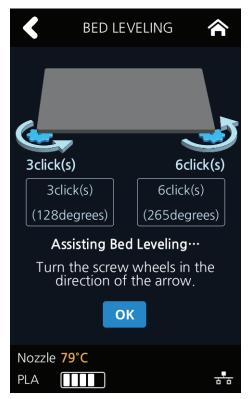
4 Turn the screw and press [OK]. The measuring is performed and the value to fix appears again.
