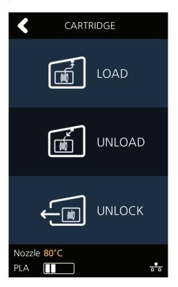
3 When [OK] is pressed at the cartridge load confirming message, cartridge load will automatically proceed. The filament reaches to the nozzle and it is heated up to the specified temperature. Then the filament is inserted into the heated nozzle. After the process has finished, screen will automatically return to the [HOME] screen.
