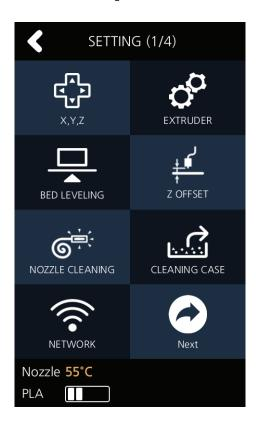
3 To Control [EXTRUDER], Nozzle temperature needs to be raised.
