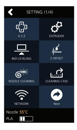
In order to get rid of all left over filament residue, the nozzle needs to be heated.
